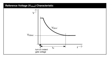
After  $t_{bl}$  has passed, the  $V_{CE}$  monitoring will be triggered as soon as  $V_{CEsat} > V_{CEref}$  and will turn off the IGBT. The error memory will be set, and the output PRIM\_HOLD\_OUT changes to the HIGH state. Possible failure modes are shows in the following pictures.
